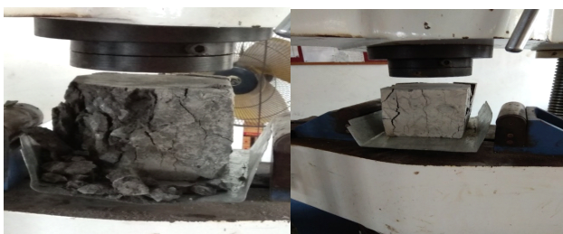
Fig. 5: Failure criteria for nominal concrete.
