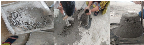
Fig. 3: Process of concrete mixing slump test.
