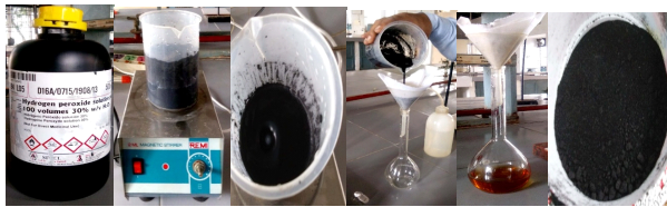
Fig. 2: Process of cleaning tyre rubber waste.
