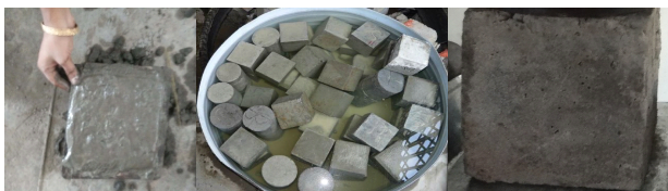
Fig. 4: Rubberized concrete cube, curing and drying for compressive strength test.
