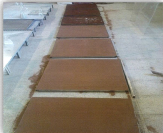
Fig. 2: Samples of soils placed into tray for test.
