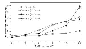
Fig. 6: Influence of nitrate nitrogen concentration by voltage under different additive amounts.
