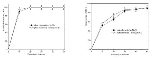
Fig. 2: The removal effect of nitrogenous compounds is shown when the electric current was constant with the electrolysis time prolonging.
