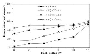
Fig. 4: Influence of total nitrogen removal by dosing under different voltages.
