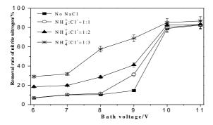
Fig. 5: Influence of nitrous nitrogen removal by voltage under different additive amounts.
