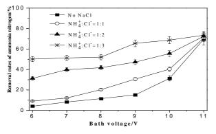
Fig. 3: Influence of ammonia nitrogen removal by dosing under different voltages.
