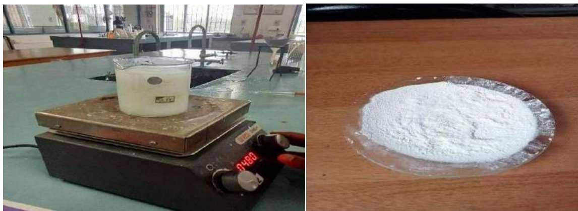
Fig. 1: a) Stirred solution of Ag-doped ZnO. b) Silver-doped zinc oxide photocatalyst powder.
