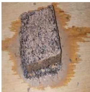
Fig. 10: Material loss during compaction of Bcp4 at m_{\text{water}} = 30 g.
