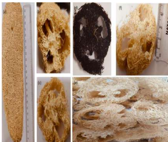
Fig. 2: (a) LS (b) cross-section of LS (c) cut piece of LS (d) alkaline, acid treated LS (e) KMnO 4 treated LS (f) SSGP-pretreated LS.
