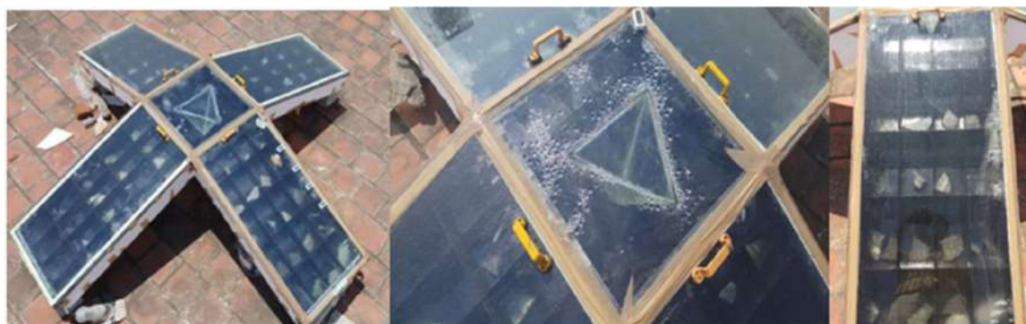
Fig. 1: Newly designed solar still.
