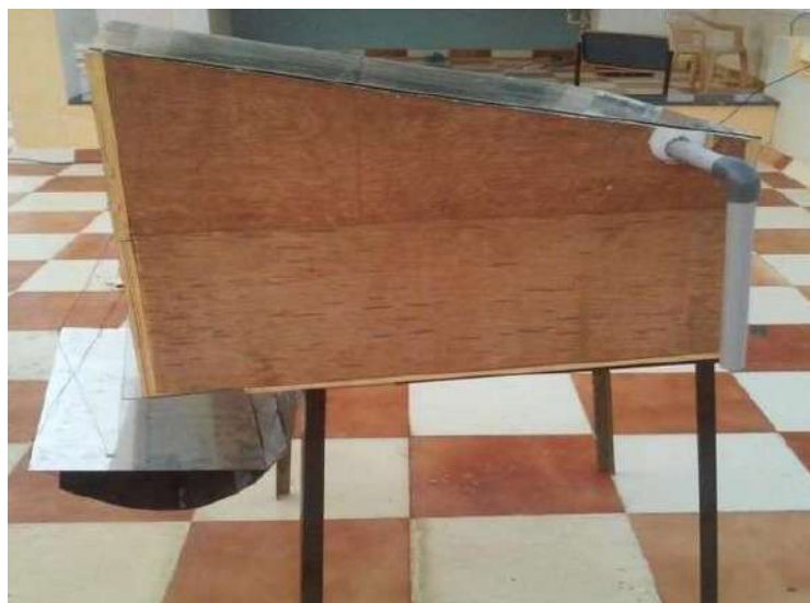
Fig. 1: Experimental setup of Solar Still.
