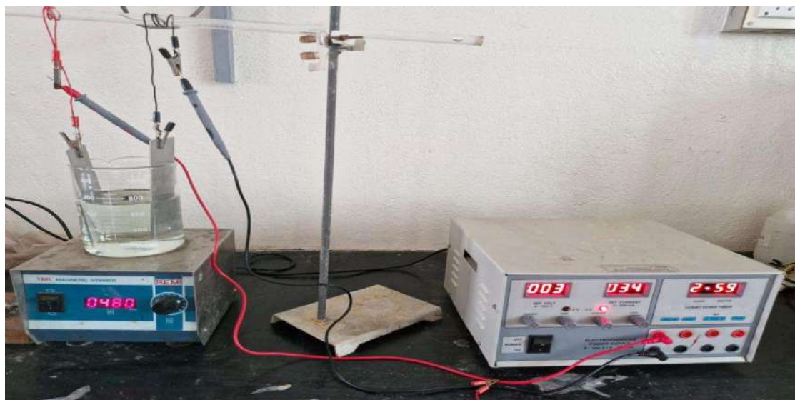
Fig. 1: Electro Fenton setup with Sacrificial stainless steel electrodes.
