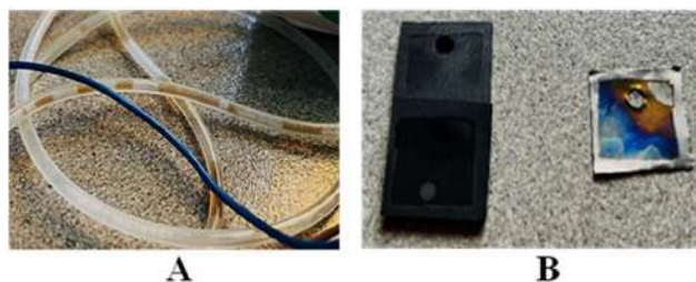
Fig. 11: Electrolyte Color Change by Metal Oxidation (A), Appearance of Graphite and Ti electrode surfaces after oxidation (B).
