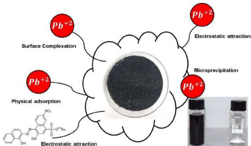
Fig. 7: Schematics of Adsorption mechanism of Pb^{+2} and EBT on JMSP AC.
