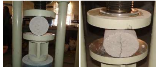
Fig. 6: Testing of cylinder specimen.
