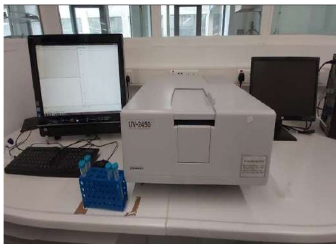
Fig. 2: Shimadzu UV-2450 double-beam UV/visible spectrophotometer.
