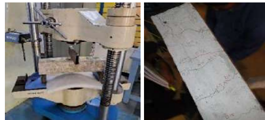
Fig. 7: Testing of beam specimen.
