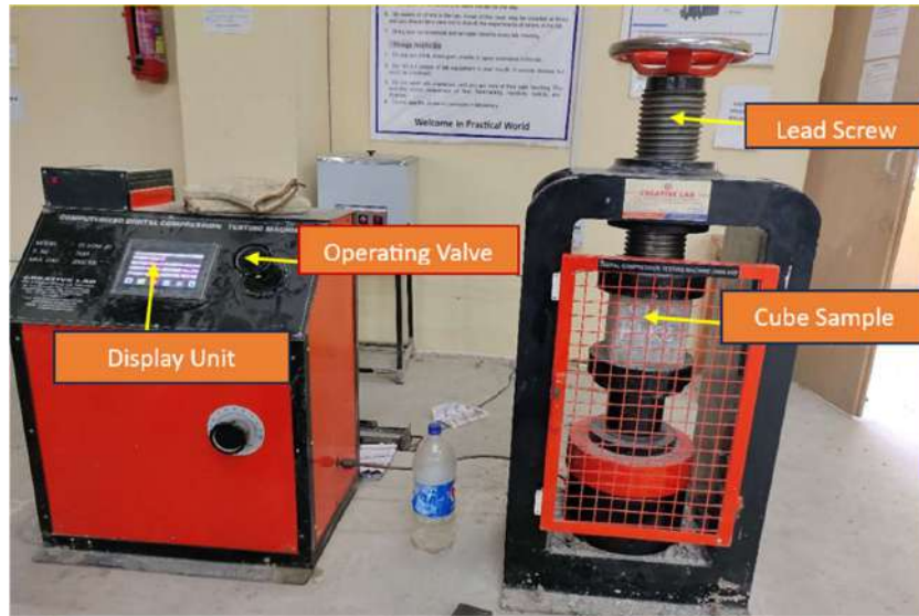
Fig. 6: Compressive testing machine used in the test experiment.
