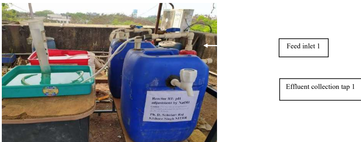
Fig. 3b: Lab-scale anaerobic reactors R1 and R2 showing feed inlets and effluent collection taps.
