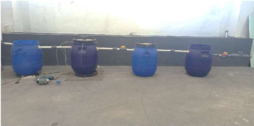
Fig. 3: Model of wastewater treatment system.
