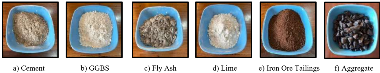
Fig. 1: Materials used to cast construction blocks
