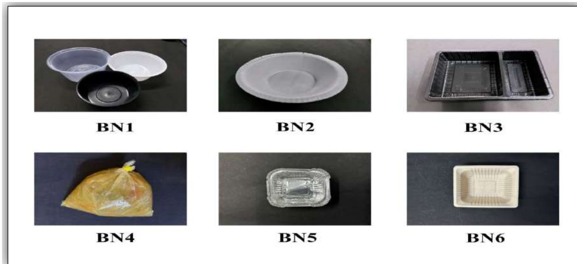
Fig. 1: BPA leaching in take-out soups from various packaging containers, with material codes assigned as: BN1 for polycarbonate (PC) plastics, BN2 for polystyrene (PS) plastics, BN3 for polypropylene (PP) plastics, BN4 for polyethylene (PE) pouches, BN5 for aluminum foils, and BN6 for areca leaf containers.
