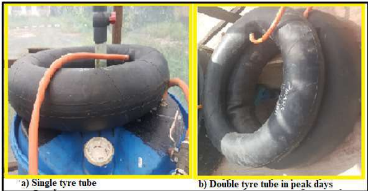
Fig. 3: Biogas-filled 175/65 R14 tyre tube.
