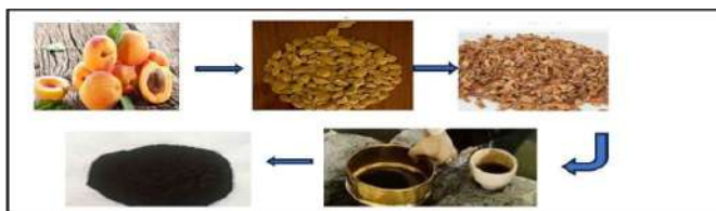
Fig. 1: Systematic presentation of biochar preparation.
