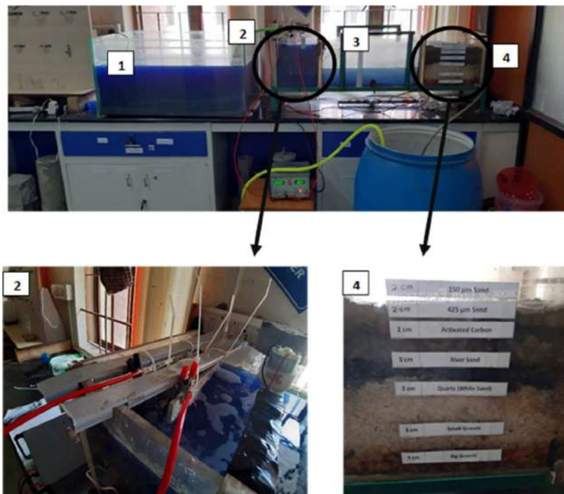
Fig. 2: Continuous Flow Reactor, Settling Tank, and Filtration.
