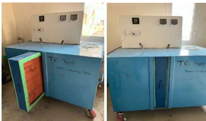
Fig. 5: Testing setup for finding Thermal conductivity of green masonry wall.
