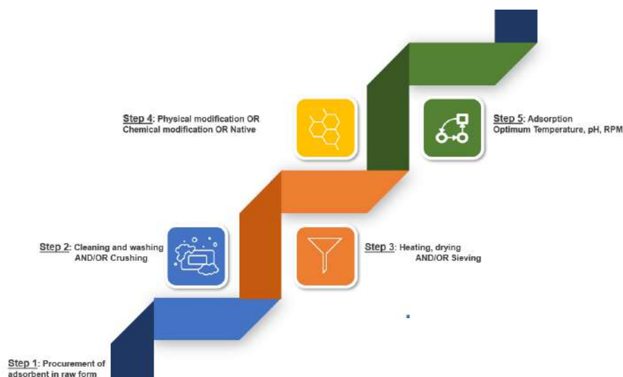
Fig. 8: Typical bioadsorbent preparation and usage cycle.
