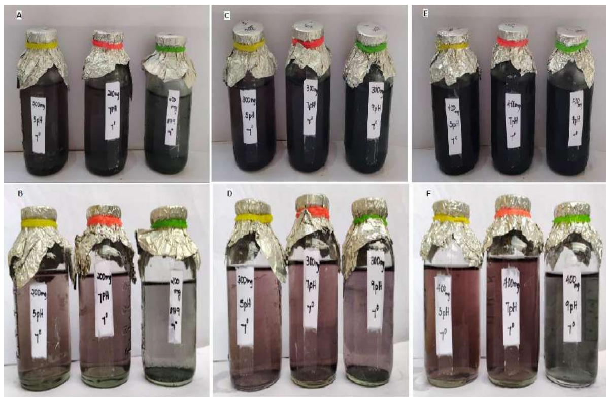
Fig. 5: photograph of dye with concentration 200 \text{ mg.L}^{-1} at 7^\circ\text{C} before (A) and after processing at pH 5, 7, and 9 (B). Photograph of dye with concentration 300 \text{ mg/L} at 7^\circ\text{C} before (C) and after processing at pH 5, 7, and 9 (D). Photograph of dye with concentration 400 \text{ mg.L}^{-1} at 7^\circ\text{C} before (E) and after processing at pH 5, 7 and 9 (F).
