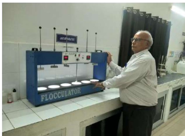
Fig. 1: Flocculator model for Jar Testing.
