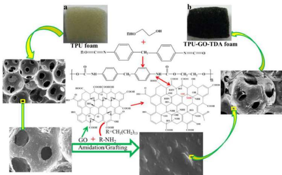
Fig. 2: Schematic illustration for the fabrication of TPU-GO-TDA foam sorbent. (Reprinted with permission from Wei et al. (2018). Copyright © 2018, American Chemical Society).
