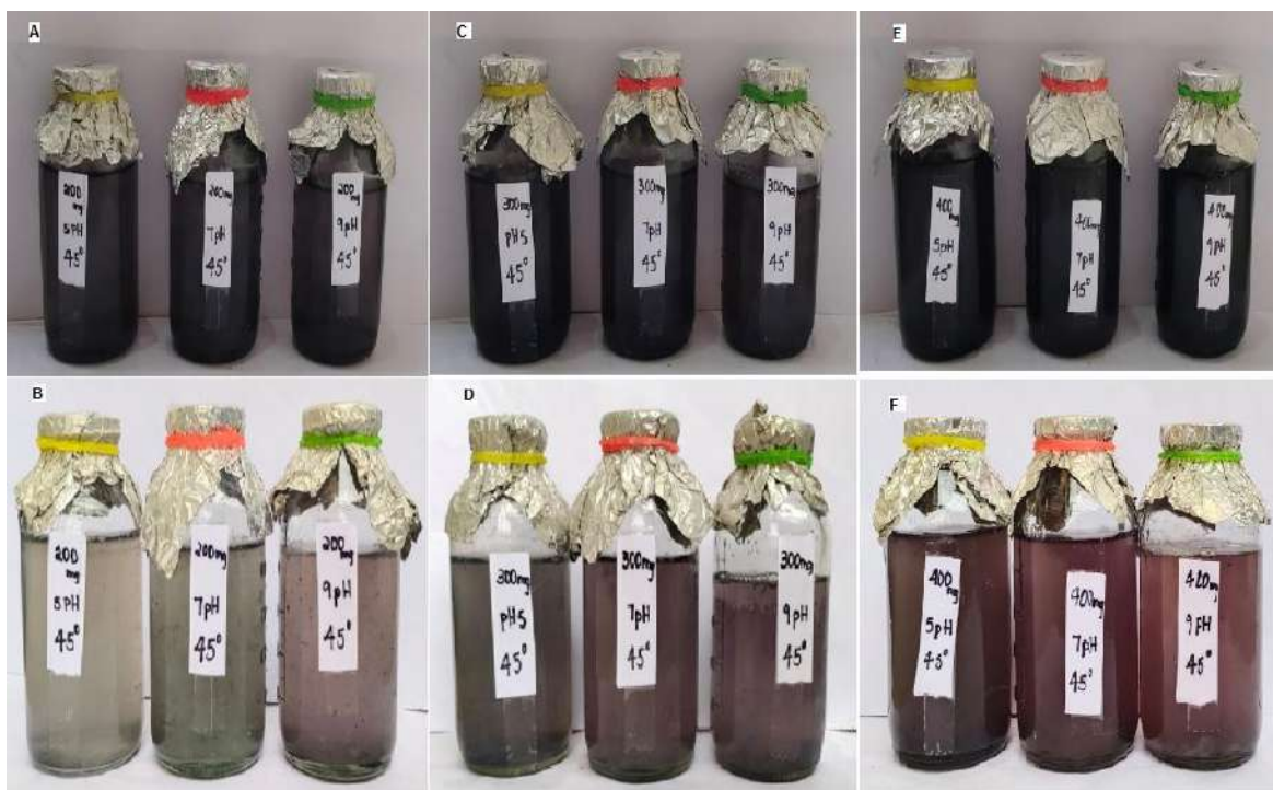
Fig. 9: Photograph of dye with concentration 200 \text{ mg.L}^{-1} at 45^\circ\text{C} before (A) and after processing at pH 5, 7 and 9 (B). Photograph of dye with concentration 300 \text{ mg.L}^{-1} at 45^\circ\text{C} before (C) and after processing at pH 5, 7 and 9 (D). Photograph of dye with concentration 400 \text{ mg.L}^{-1} at 45^\circ\text{C} before (E) and after processing at pH 5, 7 and 9 (F).
