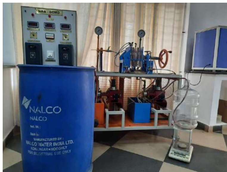
Fig. 8: Digital photograph of lab scale DCMD.
