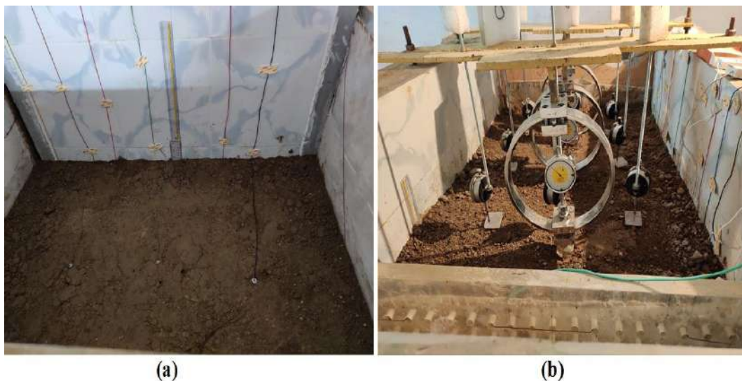
Fig. 4: Rectangular EK model image (a) Soil chamber installed with dummy electrode (b) Soil chamber with D.G. and P.R.
