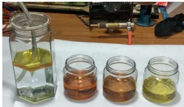
Fig. 22: Oil extraction by thermal plasma pyrolysis of Hospital plastic waste materials.
