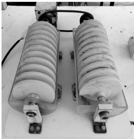
Fig. 1: Conventional biodisc system - CB (left) and spiral biodisc - SSB (right) used for stabilization of primary residual sludge.
