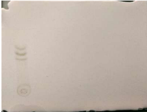
Plate 1: Lipid separation using Two mobile phases; Step 1, of 2D separation of isolate AS1-(1)
