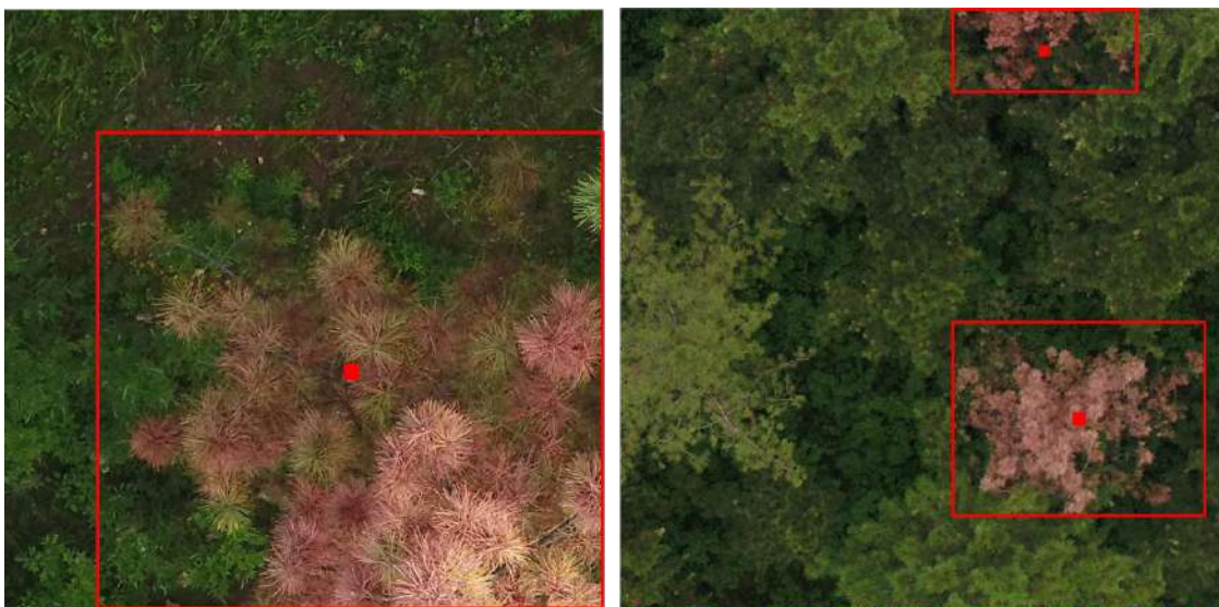
Fig. 4: Samples of the center point of the bounding box that cannot represent well of the related object.
