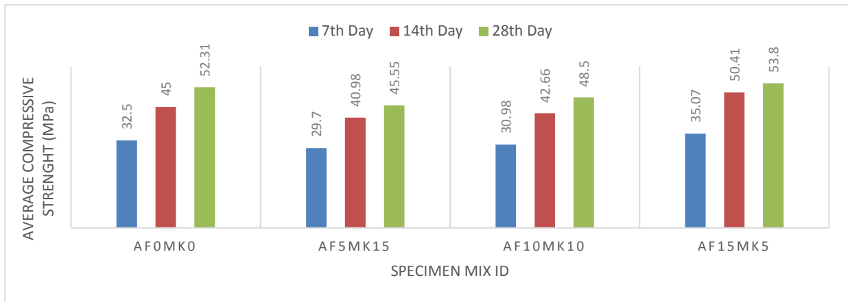
Fig 4: Comparison of Compressive strength with Ternary Blended System.
