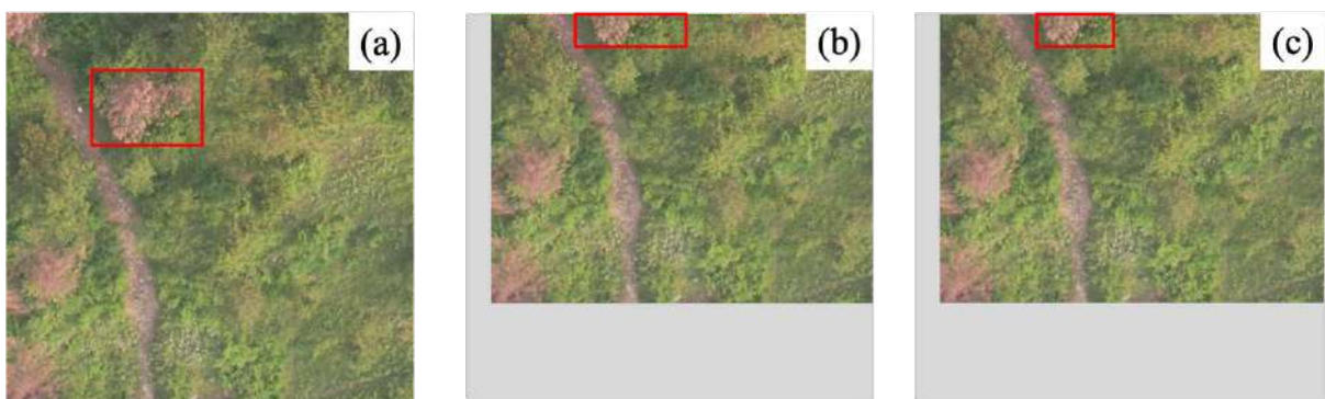
Fig. 3: (a) The original labeled picture, (b) the bounding box create in CenterNet after the affine transform, and (c) the real bounding box of the left part after the affine transform to picture.
