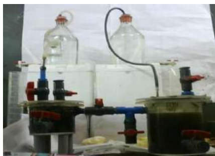
Fig. 1: Schematic representation of two-stage continuous anaerobic digester.
