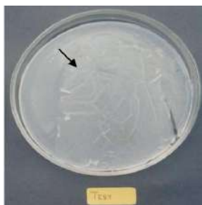
Fig. 5: Growth of strain B on polyvinyl chloride film placed on mineral salt media.
