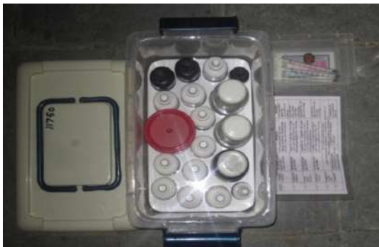
Fig. 2: TWAD Board kit for testing water samples.
