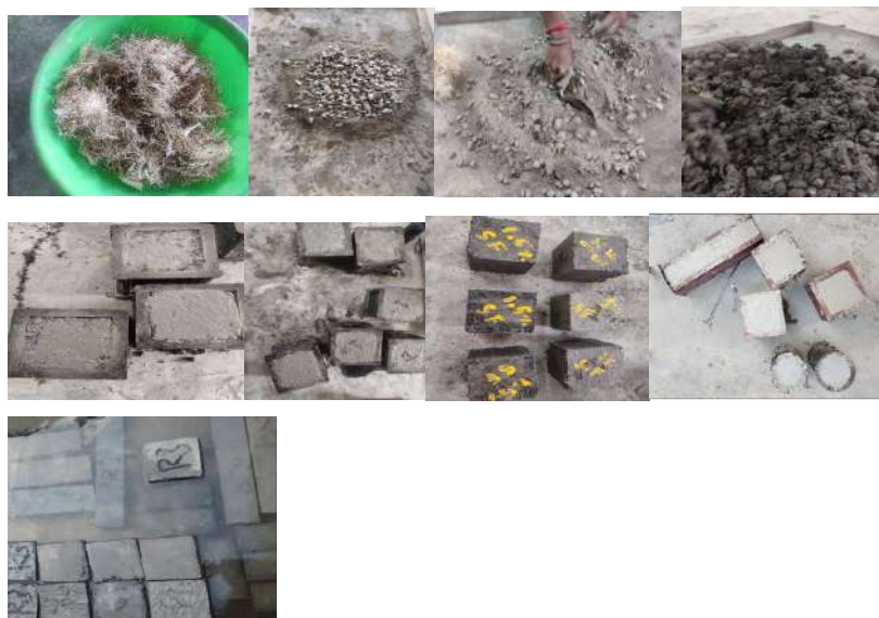
Fig. 7: Casting and curing of specimens.
