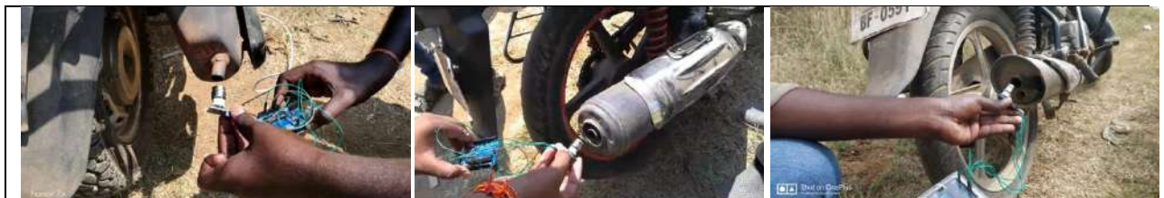
Fig. 3: Measurement of CO 2 from different vehicles.
