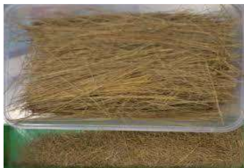
Fig. 10: Acoustic material from rice straw.
