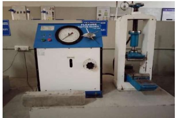
Fig. 3: Flexural strength test.
