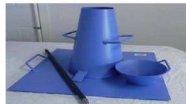
Fig. 1: Slump cone test.
