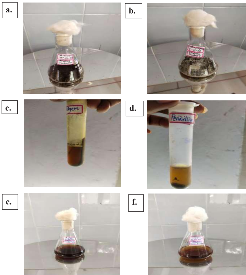
Fig. 3: a. Solid-State fermentation(SSF) of Aspergillus niger b. Solid-State fermentation of Penicillium species c. Supernatant obtained from centrifugation of filtrate from SSF of Aspergillus niger d. Supernatant obtained from centrifugation of filtrate from SSF of Penicillium species e. Crude enzyme obtained from SSF of Aspergillus niger f. Crude enzyme obtained from SSF of Penicillium species
