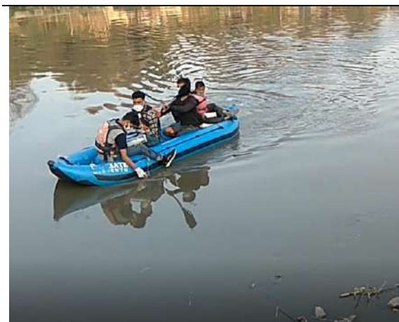
Fig. 2: Water quality data collection along Bagmati River using mobile tracing system (rafting boat loaded with measuring instrument).
