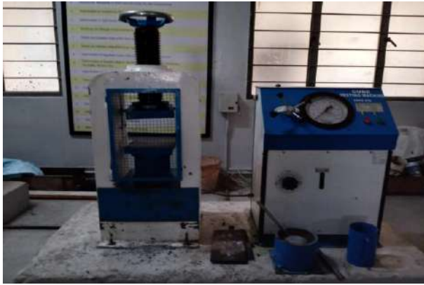
Fig. 2: Compressive strength test.
