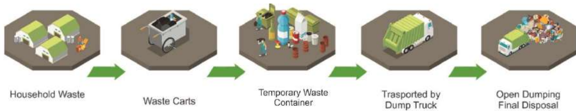
Fig. 9: Flow Diagram for existing solid waste management model.
