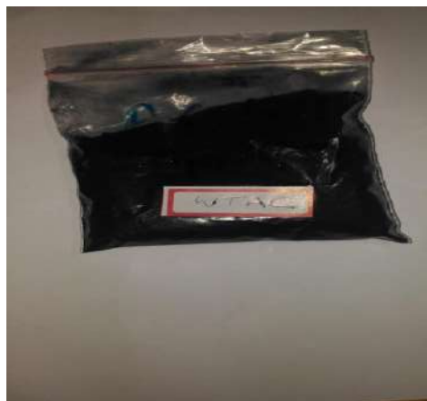
Fig. 1: Activated carbons prepared from waste tires with an average particle size of 149 μm.
