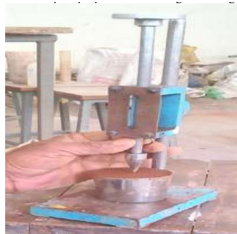
Fig. 10: Cone penetrometer used for finding the liquid limit.
