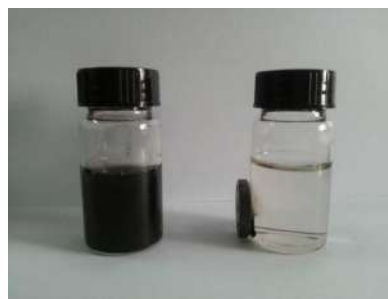
Fig. 1: The magnetic nano- \text{Fe}_3\text{O}_4 solution can easily be separated by a magnet.
