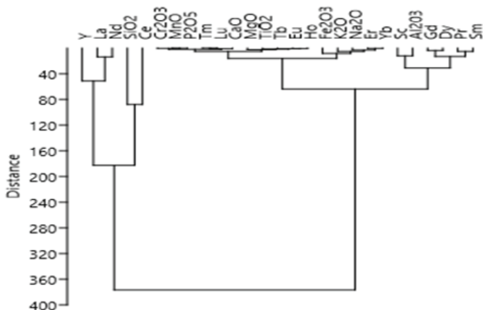
Fig.10: Dendrogram derived from the hierarchical cluster analysis of rare-earth elements and major oxides in the analysed stream sediments.
