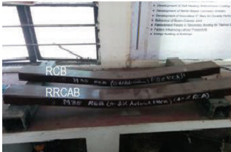
Fig. 11: Failure pattern of beams.
