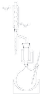
Fig. 4: Oily sludge testing device.
