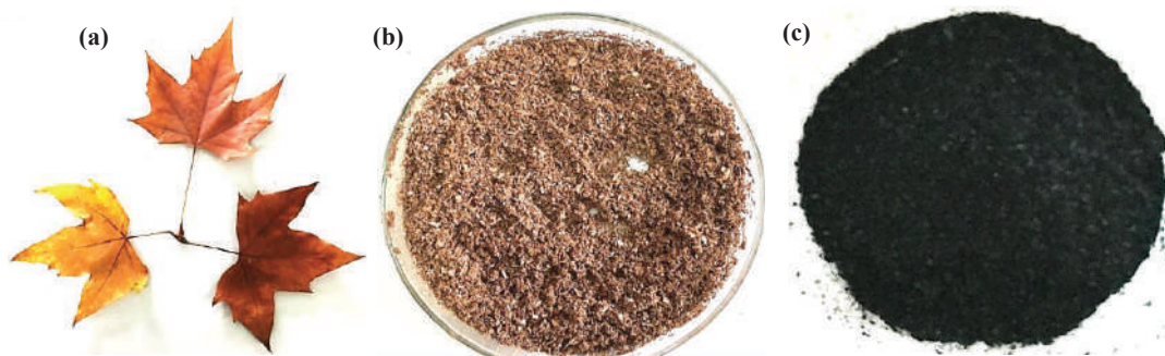
Fig. 1: (a) leaf, (b) leaf powder inoculated with H_3PO_4 and (c) activated carbon.
