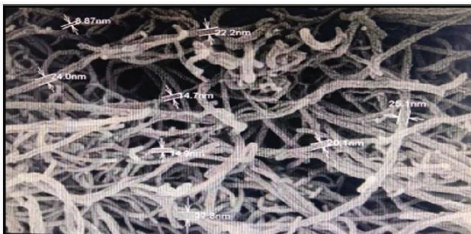
Fig. 1: TEM image of carbon nanotubes.
