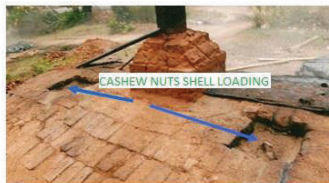
Fig. 3: Top view - Input loading cylinder with cover.
