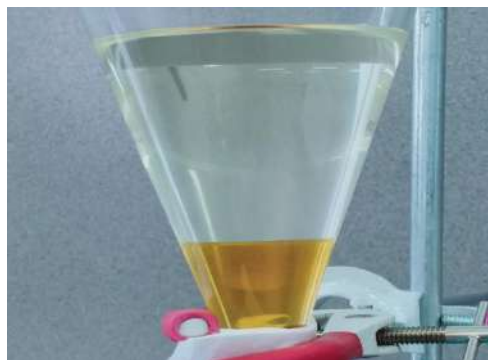
Fig. 3: Separation funnel - FAME at the upper layer and glycerine at the bottom layer.
