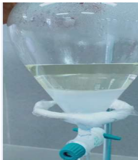
Fig. 4: Two layers after washing the FAME with distilled water 50% by FAME volume, the top layer is washed biodiesel.
