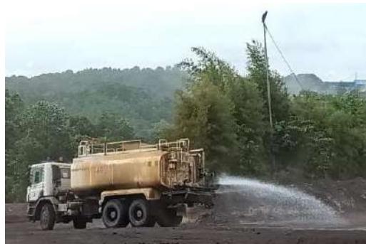
Fig. 6: Watering for mine road.
