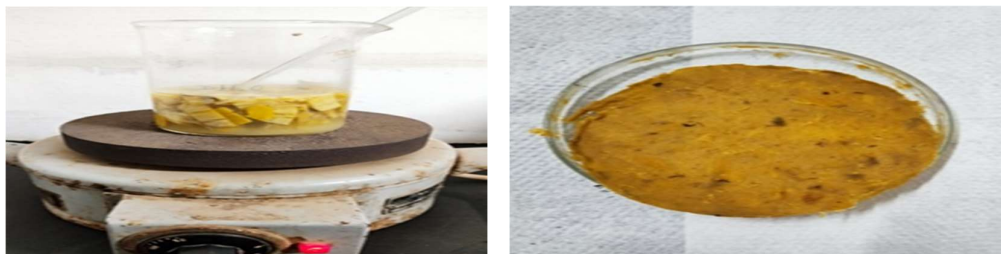
Fig. 1: Extraction of starch and production of thin, flexible bioplastic film.
