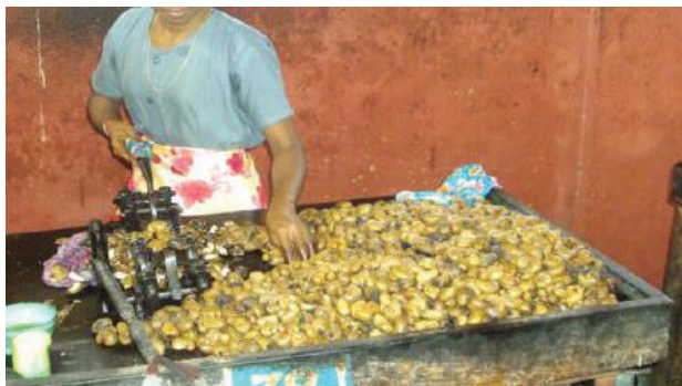
Fig. 1: Manually separating activity for cashew kernel and shells.
