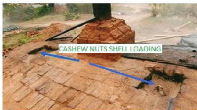
Fig. 3: Top view - Input loading cylinder with cover.
