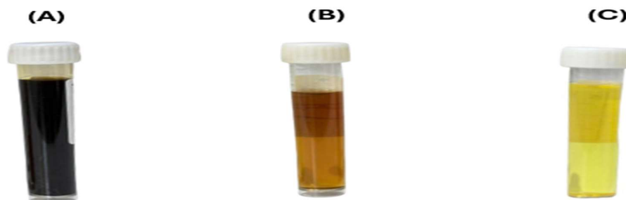
Fig. 8: (A) spent oil, (B) recovered base oil after bleaching, (C) Stock 60.
