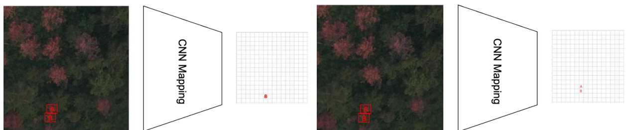
Fig. 2: (a) Two coincide center points on features from two close objects, (b) SOCP operation to two coincide center points on the feature map.
