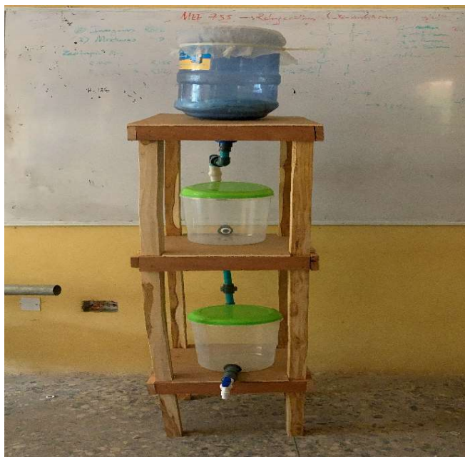
Fig. 12: Model of the stormwater treatment system.
