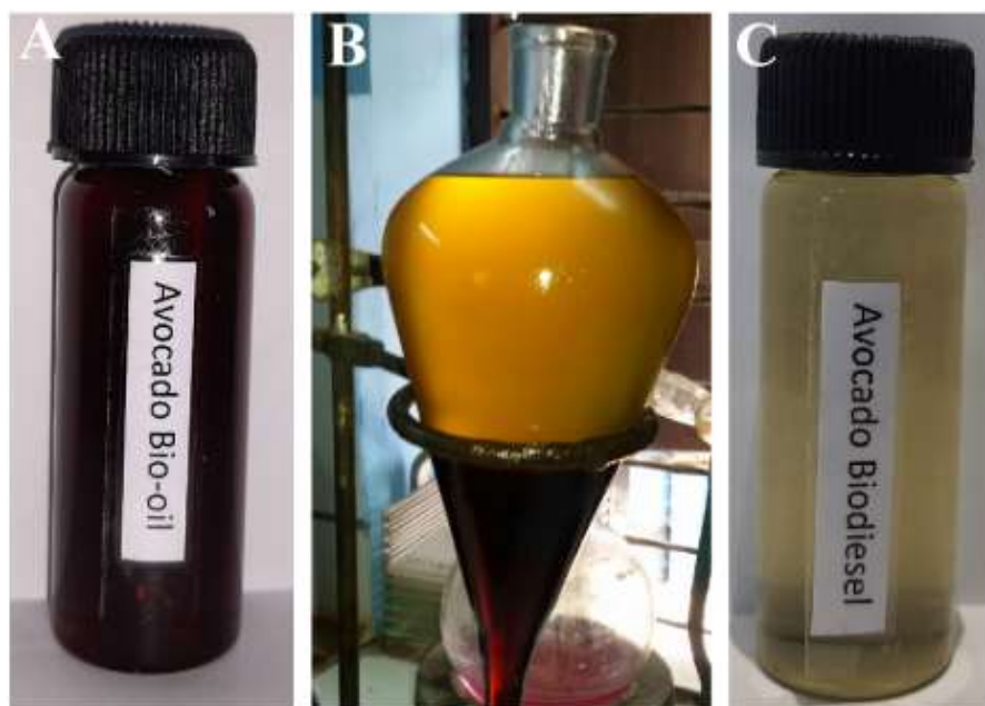
Fig. 2: Persea americana (Avocado) bio-oil (A), Transesterification (B) and Biodiesel (C).
