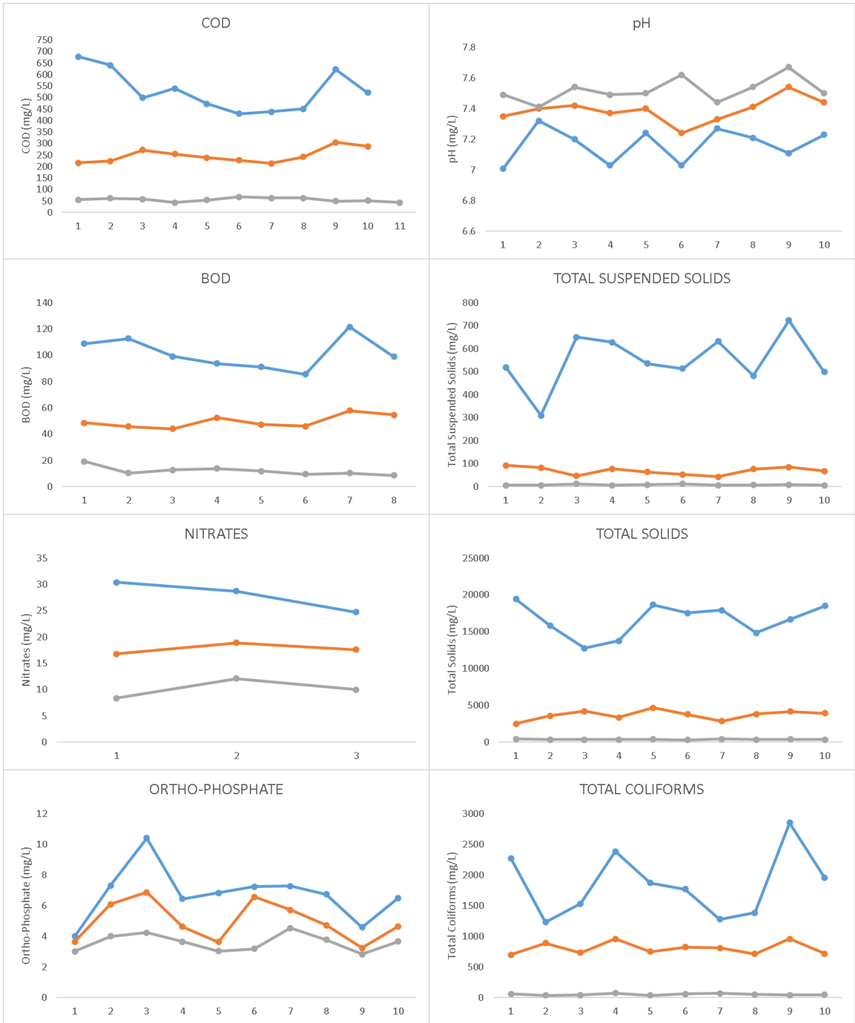
Fig. 2: Graphical representation of variation in physico-chemical parameters after each stage of treatment. The blue line indicates the inlet wastewater, orange line indicates the wastewater after anaerobic filter and the grey line indicates the wastewater characteristics after VFCW
