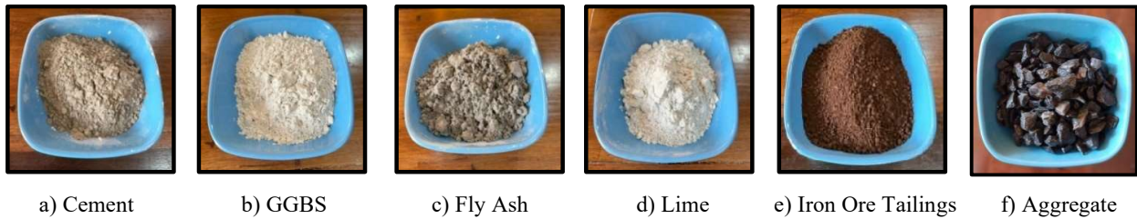
Fig. 1: Materials used to cast construction blocks
