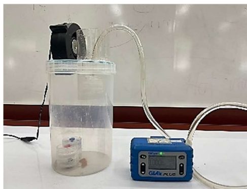
Fig. 2: Particulate matter filtration efficiency testing equipment.
