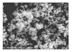
Fig. 3: SEM images of zinc oxide nanoparticles.
