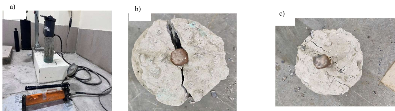
Fig. 6: a) Pull-out test, b) Uncoated samples, c) Coated samples.
