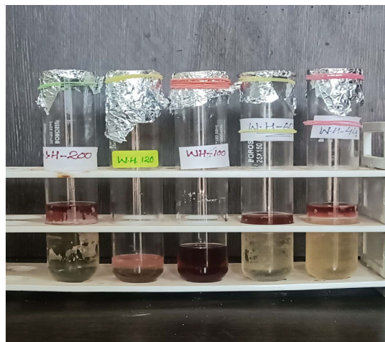
Fig. 4: Water Hyacinth treatment samples for engine oil.
