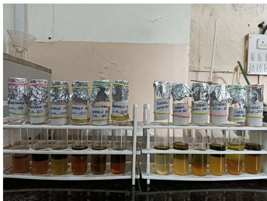
Fig. 6: Water hyacinth treatment samples for vegetable oil and diesel.
