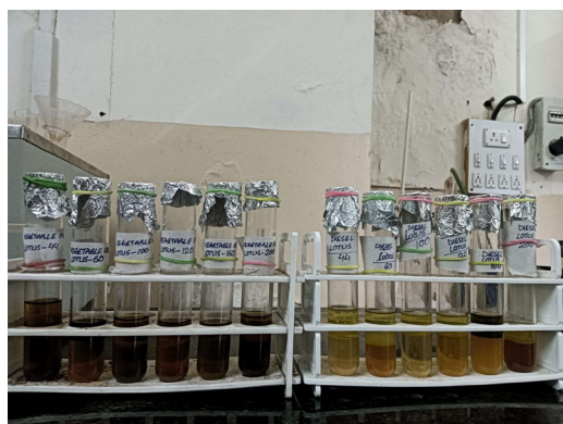
Fig. 7: Lotus treatment samples for vegetable oil and diesel.
