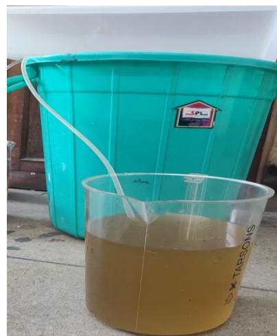
Fig. 5: Washed sludge dewatering by siphoning.
