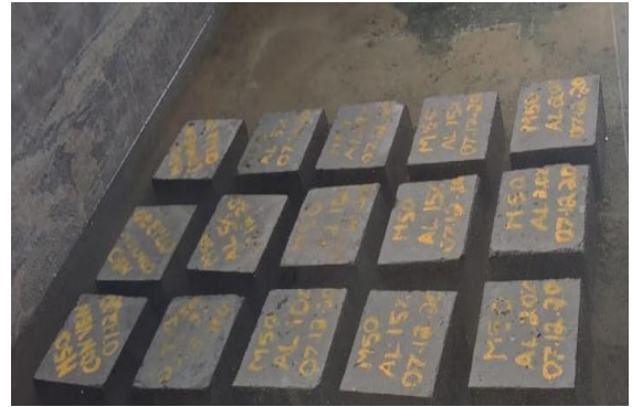
Fig. 2: Casting and curing of concrete specimen.
