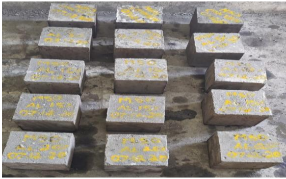
Fig. 2: Casting and curing of concrete specimen.
