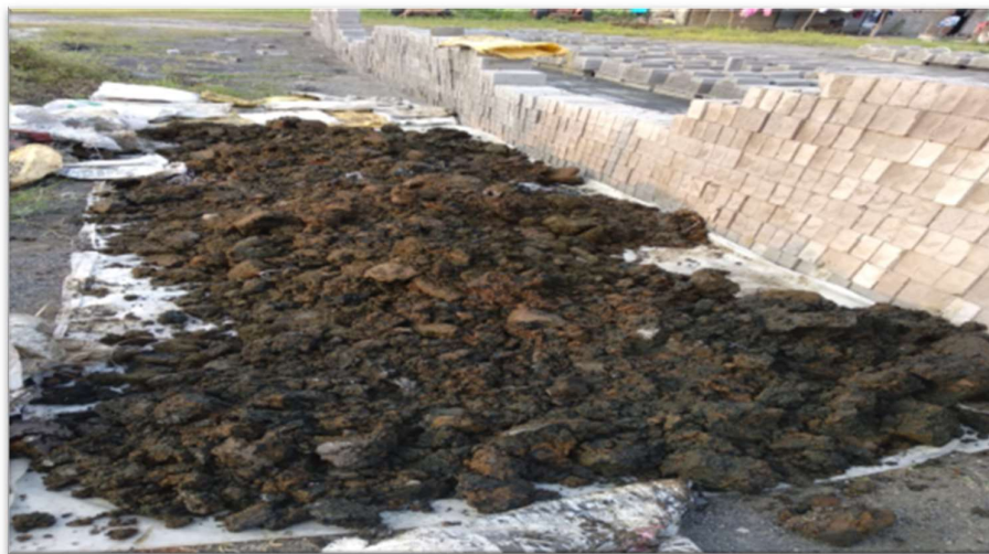
Fig. 2: Open-air drying of wet sludge.
