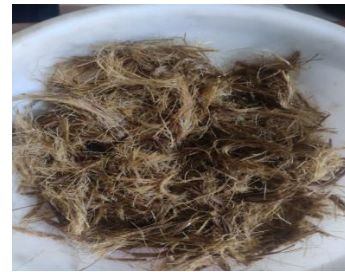
Fig. 6: After 10 days fiber immersed in Na 2 CO 3 .
