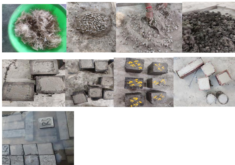
Fig. 7: Casting and curing of specimens.
