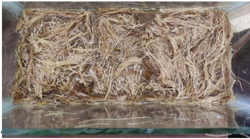
Fig.5: Sisal fiber immersed in Na 2 CO 3 solution.
