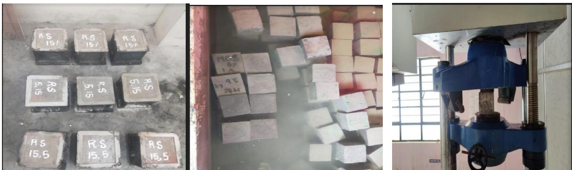
Fig. 2: Casting, curing, and testing of concrete specimen.
