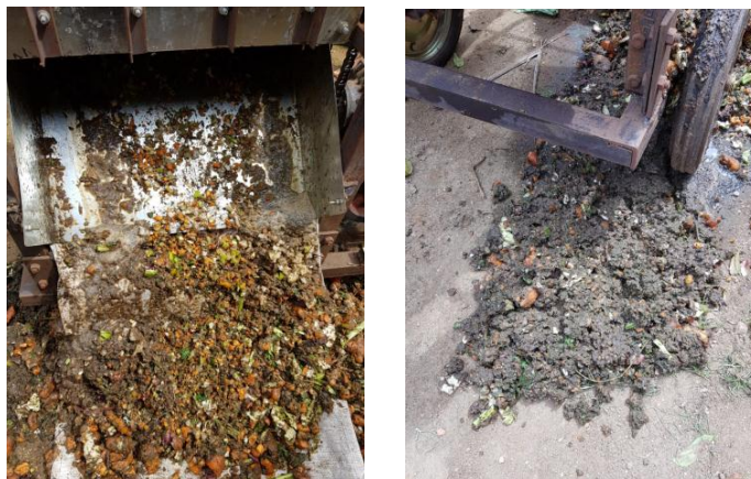
Fig. 8: Vegetable waste shredded using the machine (Left- first trial, Right- Second trial)
