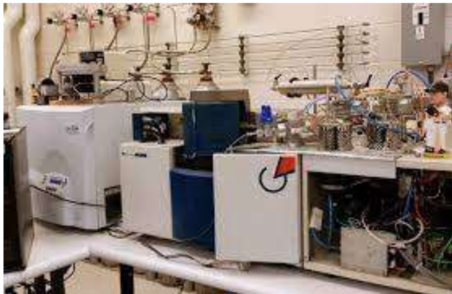
Fig. 5: Isotope ratio mass spectrometer (Isoprime, Micro mass, UK) (George & Gerogios 2020).
