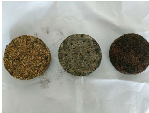
Fig. 5: Paddy Straw, Coconut Coir, and Waste Paper Panel (100 Mm).
