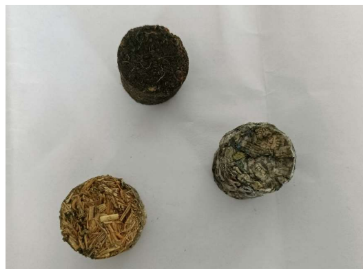
Fig. 6: Paddy Straw, Coconut Coir and Waste Paper Panel (30 Mm).
