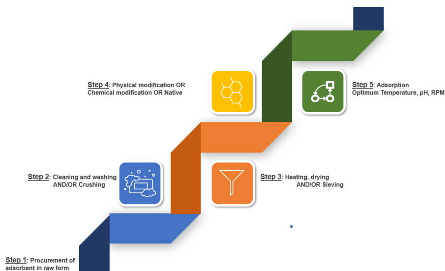
Fig. 8: Typical bioadsorbent preparation and usage cycle.
