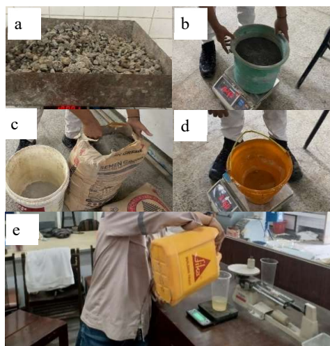
Fig. 1: Materials used in this study: (a) coarse aggregate; (b) fine aggregate; (c) cement; (d) water; (e) superplasticizer.
