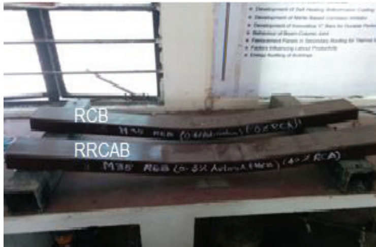
Fig. 11: Failure pattern of beams.
