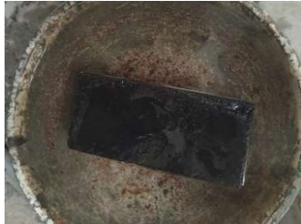
Fig. 9: Water absorption test.
