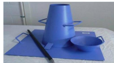
Fig. 1: Slump cone test.
