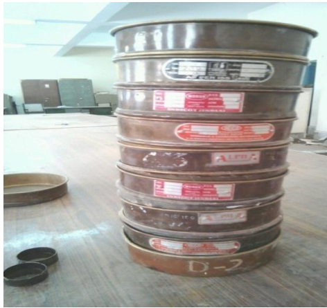
Fig. 7: Sieve set used for particle size analysis.
