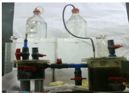
Fig. 1: Schematic representation of two-stage continuous anaerobic digester.
